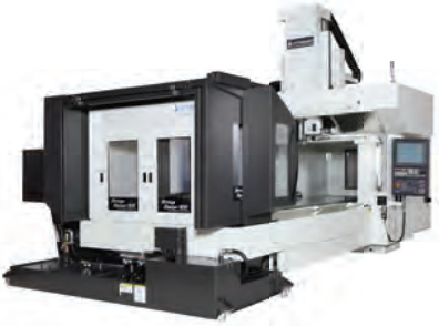
Bridgecenter-10G Eksen Hareketleri: 100" x 64" x 32" (2,540 x 1,615 x 800 mm)
